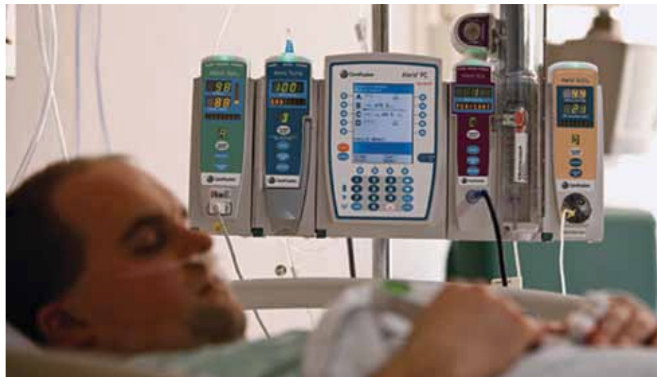
Figure 2. Modular IV medication safety system with PCA pumps and pulse oximetry and capnography monitors on a common technology platform. Source: CareFusion, San Diego, CA. Used with permission.
